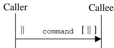
Figure 13 - An Opaque Asynchronous Interaction Pattern, returning no completion information.
